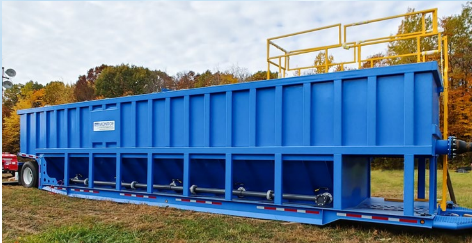
The X-Flo Mobile Clarifier was able to effectively reduce TSS at flows of approximately 500 GPM
