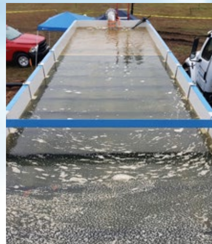
Clear water in X-Flo plate separator section
