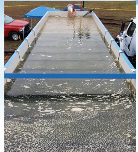
Clear water in X-Flo plate separator section
