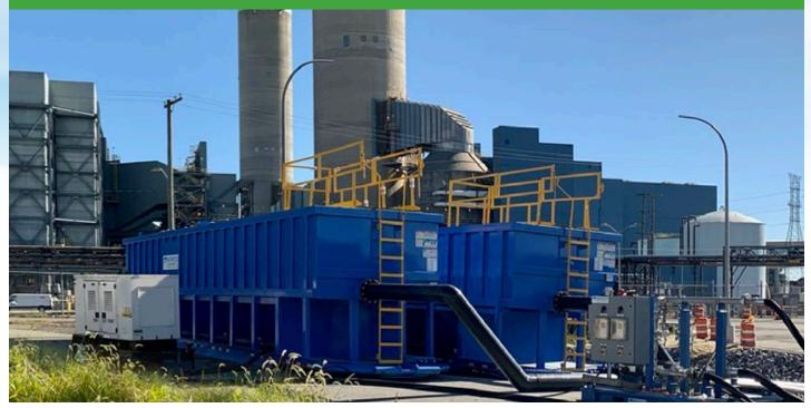
Monroe X-Flo Mobile Clarifiers operating at a coal-fired power plant. The X-Flo Clarifiers have become a favorite at this site, most notably for their ease of installation and ability to treat high liquid volumes in a short time. In this instance, the plant was executing a wash down during a planned outage and needed to separate fly ash from the wash liquid. The Monroe X-Flo Mobile Clarifiers and Monroe Sludge Pump Skid are treating a combined flow of 2,000 GPM.
