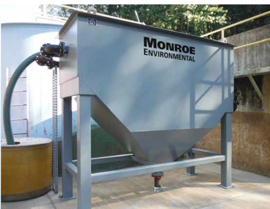
Horizontal Clarifier pilot
