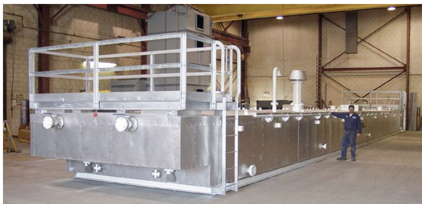
14 ft. x 90 ft. long 105 GPM API Separator with cover, mineral wool insulation, and aluminum cladding. The unit shipped from our factory fully assembled.
