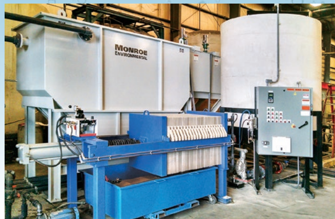
Turnkey Horizontal Clarifier system with pumps, piping, sludge holding tank, filter press, and controls
