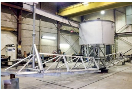
46 ft. diameter stainless steel Circular Clarifier fully assembled in Monroe shop
