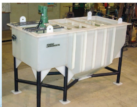
40 GPM Horizontal Clarifier with full polypropylene construction for treating low pH plating wastewater
