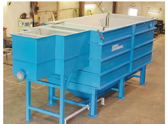
300 GPM Horizontal Clarifier for truck wash facility fully assembled in Monroe shop
