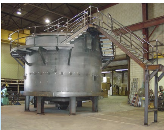
18 ft. steel tank Circular Thickener for an industrial steel manufacturer fully assembled in Monroe shop
