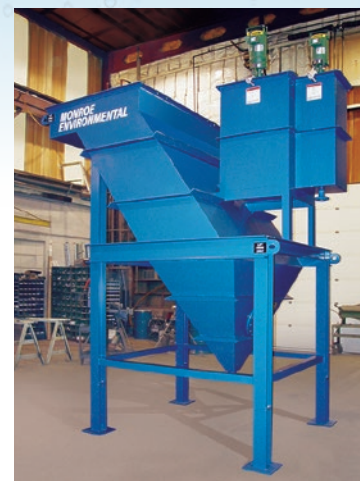
Vertical Clarifier fully assembled in Monroe shop
