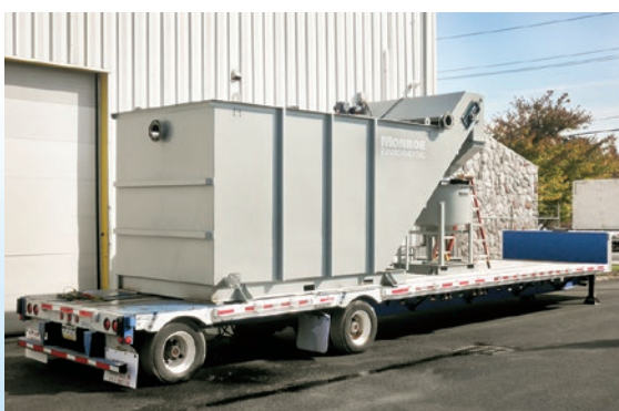
200 GPM Horizontal Clarifier with drag conveyor, truck mounted for portable treatment of hydraulic fracturing water
