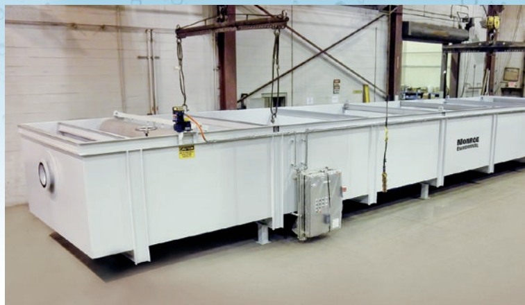
900 GPM API Separator, mild steel construction with drag conveyor, screw conveyor, pipe skimmer, and oil roll. The unit, measuring 60 ft. long x 12 ft. wide x 8 ft. high, shipped from our factory fully assembled.
