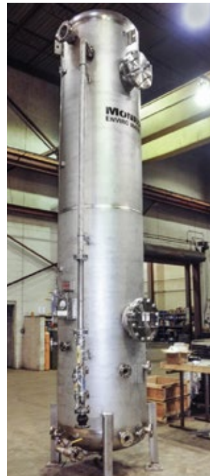
H 2 S Scrubber for syngas conversion using an amine scavenger scrubbing liquor with irrigated packing. The required H 2 S removal was over 99.98% to ensure a high-purity, low-sulfur final product. The unit was designed for 1,500 SCFM @ 120°F.
