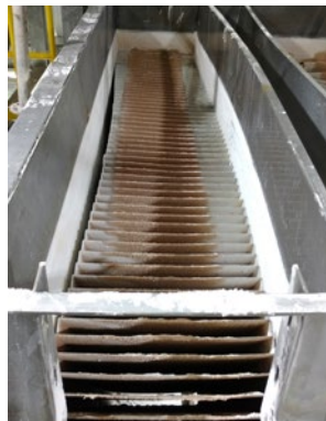
Before: Lamella plate clarifier with internal components that were warped, buckling, and in danger of collapsing.
