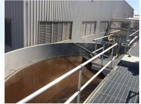
45 ft. diameter Circular Thickener on legs with tank, supports, drive mechanism, bridge, sludge rakes, skimming system, and piping for wastewater treatment at a gypsum plant
