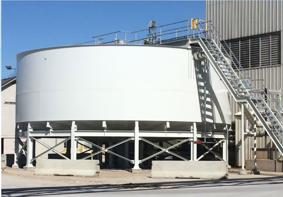
45 ft. diameter Circular Thickener on legs with tank, supports, drive mechanism, bridge, sludge rakes, skimming system, and piping for wastewater treatment at a gypsum plant
