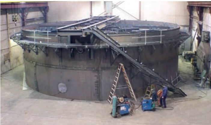
Circular Oil/Water Separator for primary treatment of waste oils and solids at a steel mill. The 50 ft. diameter clarifier was designed with low sidewater depth, inlet diffusion, and multiple skimming arms and collection troughs for enhanced oil removal.
