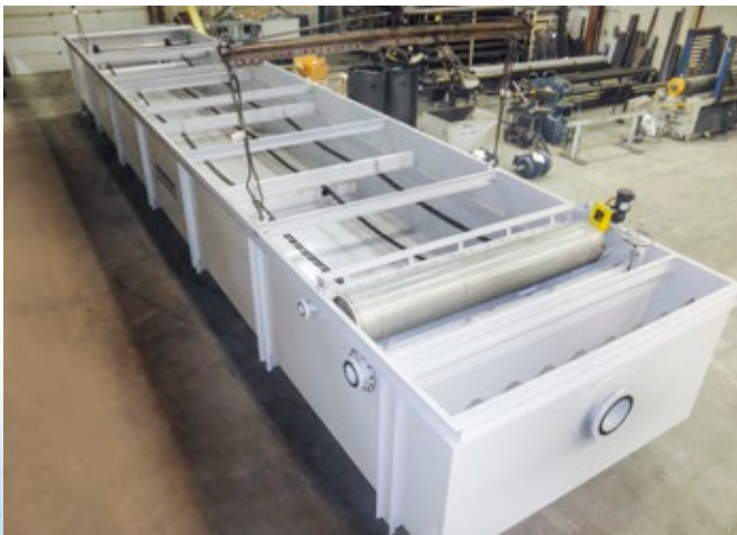
900 GPM API Separator for free oil separation prior to a DAF. The system featured inlet diffusion reaction jet baffles, chain and flight conveyor, and customized oil skimming system with collection beach and auger trough.
