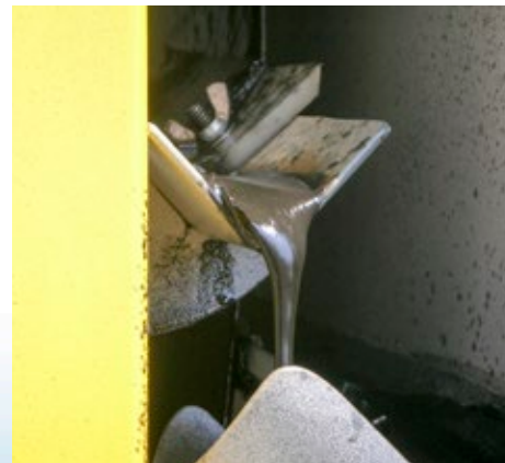
Monroe 8A Belt Skimmers for oil recovery from wastewater tanks at a steel mill. The custom thermoplastic belt was rated to withstand 180°F liquid temperatures.
