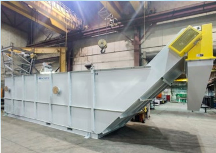
Drag tank for mill scale separation for steel tube mill. Chain and flight drag conveyor to capture and remove solids from mill water and a tube skimmer to remove floating oil. The system is rated for 660 GPM.
