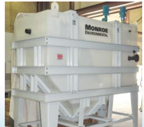
40 GPM Horizontal Plate Clarifier to remove TSS from pickling wastewater prior to membrane filtration. The polypropylene clarifier was equipped with chemical mixers, HDPE separation plates, and surface oil skimmer.
