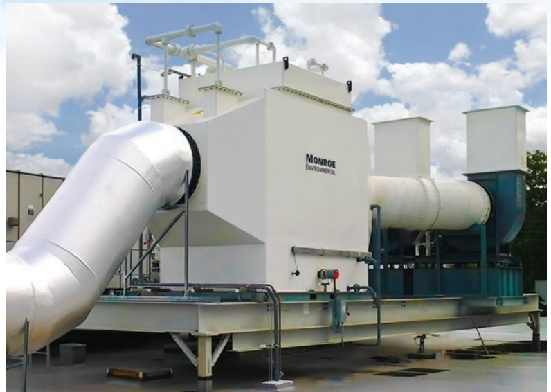
30,000 CFM Horizontal Packed Bed Scrubber with polypropylene construction to remove chemical fumes emitted from acid-dip tanks at a semiconductor manufacturing facility.
