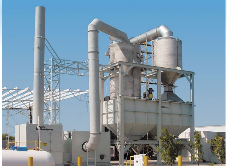
20,000 CFM Multi-Stage Scrubbing System for solid waste incineration process. (From right): Ceramic-lined inlet duct, rapid water quench, adjustable Venturi Scrubber, liquid clarification tanks, Packed Bed Scrubber, and Carbon Adsorber.
