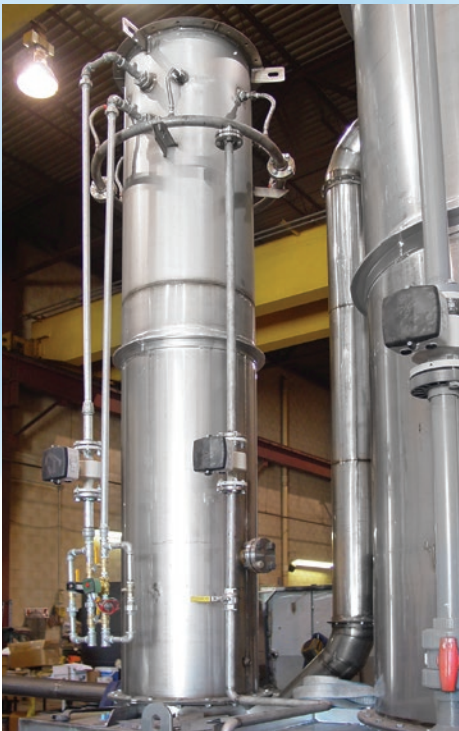
High temperature and corrosion resistant evaporative Quench Tower
