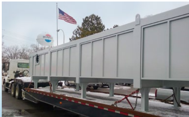
420 GPM API Separator for wastewater treatment at a biorefinery. The system included a chain and flight conveyor and oil roll + pipe skimmer for oil removal. The separator is designed to remove free solids and oil prior to a DAF.
