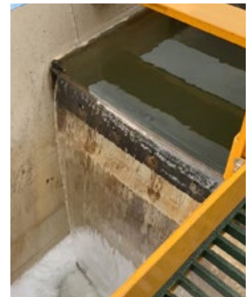
Monroe X-Flo Mobile Clarifier™ for treatment of wastewater (produced water, drilling mud, etc.) from oil and gas hydraulic fracking operations. System provided TSS removal and oil/water separation for 300 GPM flow.
