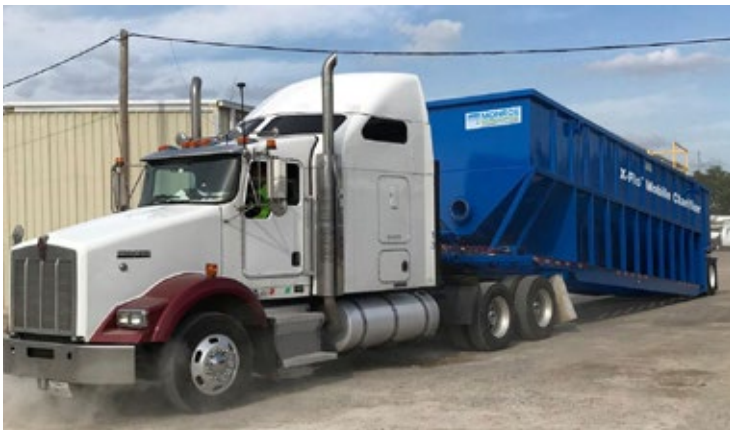
X-Flo Mobile Clarifier™ deployed for temporary treatment of produced water at a fracking well. The X-Flo Clarifier replaced multiple weir tanks with a single unit and outperformed other separators.
