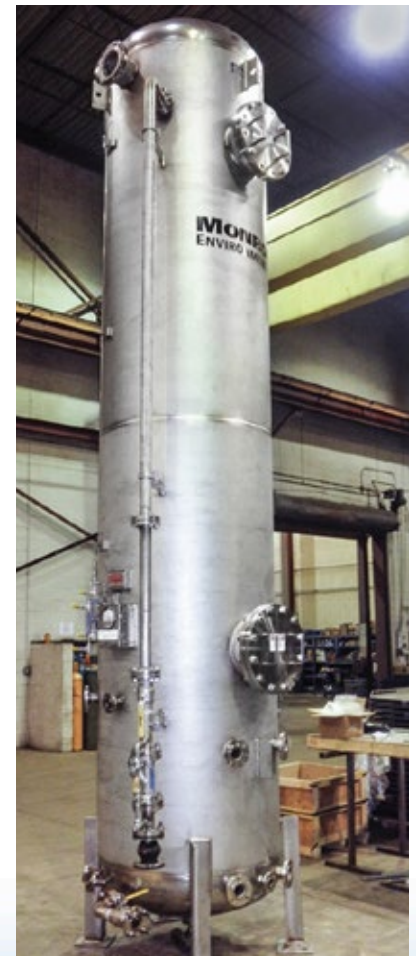
1,500 ACFM Packed Tower Scrubber to remove H 2 S from syngas conversion process at a biodiesel plant. Unit was built and stamped to ASME VIII code; 316L SS construction.
