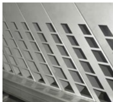
Influent Flow Distributors
