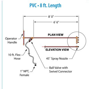
**Monroe Environmental**® has developed a very effective tool for removing solids and debris accumulated on the separator plates of lamella-style inclined plate clarifiers: **The Monroe Plate Cleaning Wand**. This product has been developed as part of our continued effort to improve operations and maintenance for your plant, and is the perfect compliment to our top of the line Vertical Plate Clarifiers.
