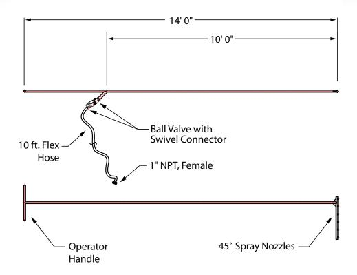
**Monroe Environmental®** has developed a very effective tool for removing solids and debris accumulated on the separator plates of lamella-style inclined plate clarifiers: **The Monroe Plate Cleaning Wand**. This product has been developed as part of our continued effort to improve operations and maintenance for your plant, and is the perfect compliment to our top of the line Vertical Plate Clarifiers.
