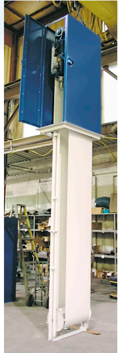
Oil Recovery Unit
