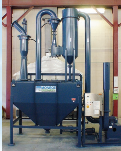
Left: 1,000 CFM Scrubbing System to remove lime dust from a chemical manufacturing process. (From left): Ejector Venturi, liquid clarification tank, high energy Venturi Scrubber, and cyclonic separator. The unit was designed to achieve 95% efficiency on 0.5 micron particles
