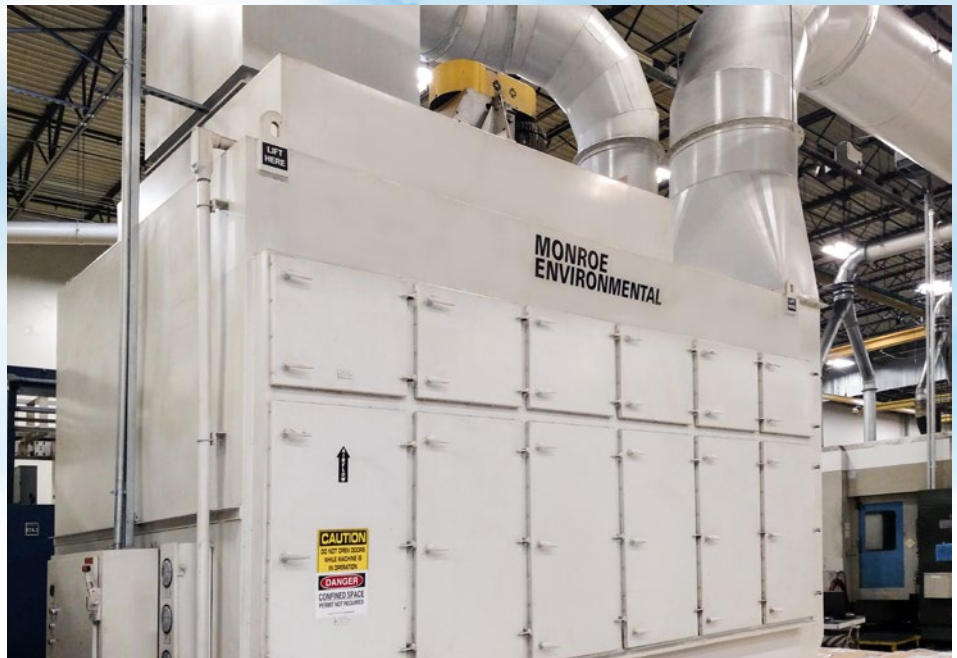
Multi-Stage Mist Collector at an engine machining plant
