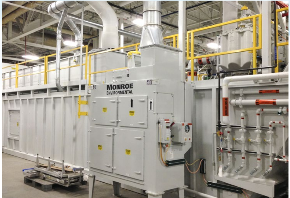
Mist Collection system exhausting machining operations at an automotive plant
