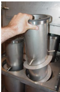
Spiral tubes are easy to remove, no hand tools required.
