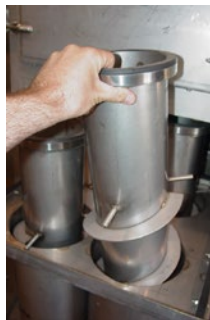
Spiral tubes are easy to remove, no hand tools required.
