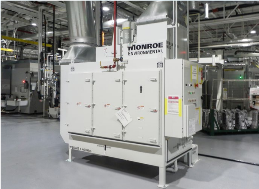
Left: Machining exhaust using Multi-Stage Mist Collector media filtration, Right: 7,000 CFM Multi-Stage Mist Collector during final assembly at Monroe shop
