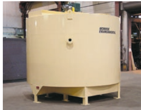
10 ft. diameter Circular Clarifier to remove clay fines from wastewater at a minerals plant. System was designed to remove 82 lb/hr of solids from 100 GPM flow.
