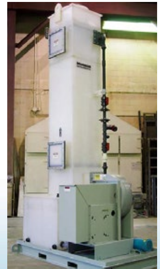
1,350 CFM Polypro Packed Tower Scrubber with 60 ft. discharge stack to remove HCl from acid tank vent at gold mine.
