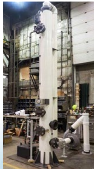
300 CFM Packed Tower Scrubber to remove HCl fumes from operations at a magnesia plant using water only.
