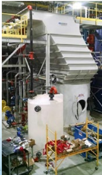
Monroe X-Flo Mobile Clarifiers™ for water treatment train at a sand mine. Units were custom built to allow up to 12,000 GPM max hydraulic flow.
