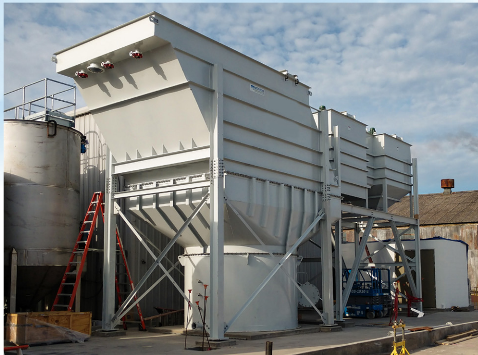
750 GPM Vertical Plate Clarifier with three pretreatment mixing tanks and integral sludge thickener to clarify process water at specialty insulation manufacturing plant. The system was purchased as a result of the successful pilot study.
