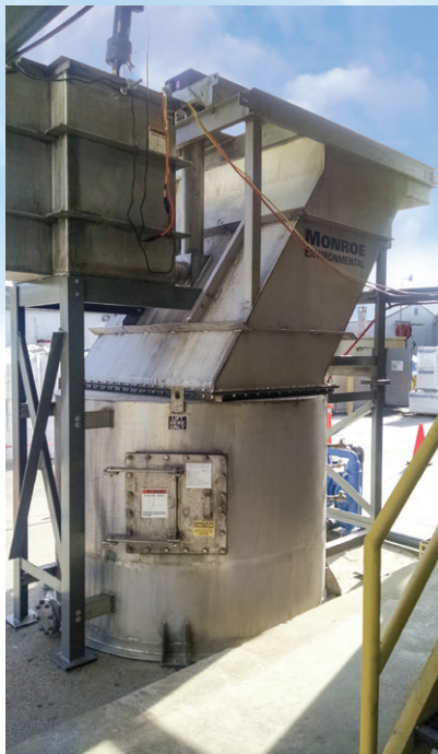
50 GPM Vertical Plate Clarifier Rental Pilot System used to trial an improved clarifier technology prior to full scale investment.
