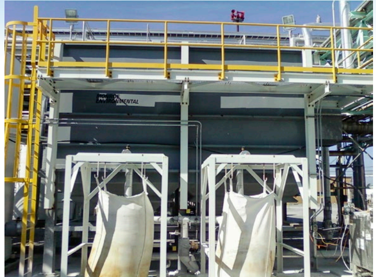
600 GPM Horizontal Clarifier with dual pyramid hoppers
