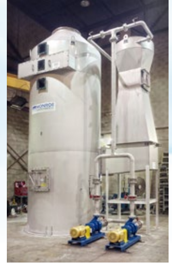
27,000 ACFM Monroe Multi-Stage Scrubbing System with Venturi Scrubber and Cyclonic Separator to remove particulate from food dryer exhaust prior to VOC destruction with a regenerative thermal oxidizer.
