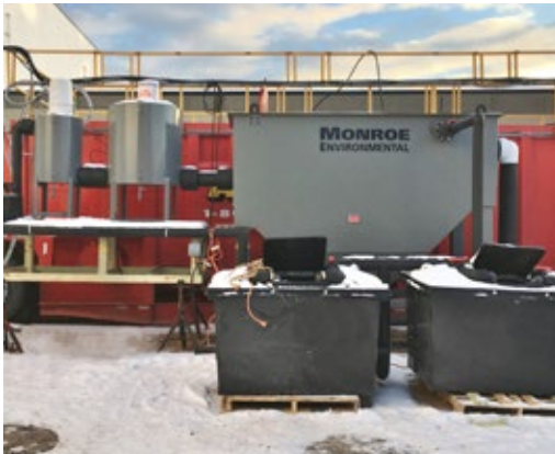
50 GPM Horizontal Clarifier pilot system for a waste stream from the production of fried foods as well as the plant's sanitary waste. The system was chosen due to its ability to separate both floating and settleable solids.
