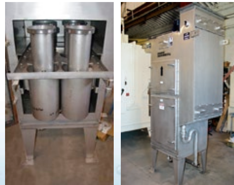
1,000 ACFM Spiral Tube Mist Collectors for mist collection from cheese mold wash-down/cleaning process. The spiral tubes provide a high level of mist agglomeration and removal without using filters.
