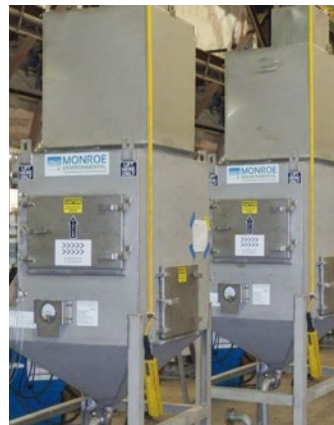
2,000 ACFM Dual Throat Venturi Scrubbers , 304 SS construction for particulate collection from marshmallow powdered sugar coating operation.
