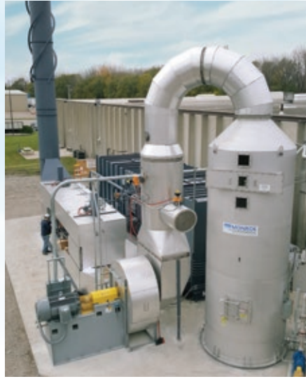
27,000 ACFM Monroe Multi-Stage Scrubbing System with Venturi Scrubber and Cyclonic Separator to remove particulate from food dryer exhaust prior to VOC destruction with a regenerative thermal oxidizer.
