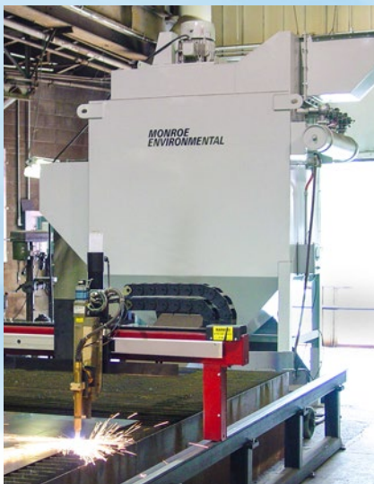
5,000 CFM Cartridge Dust Collector to capture exhaust from CNC plasma cutting operation
