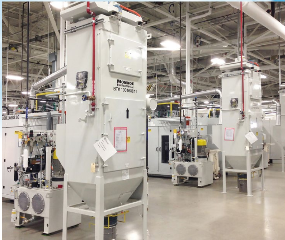
Monroe Cartridge Dust Collectors equipped with fire suppression systems operating in the field
