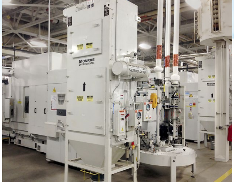
Cartridge Dust Collection system exhausting machining operations at an automotive plant
