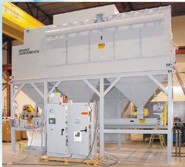
Custom configurations, including ceiling or roof designs, are available where a standard collector cannot be used. 30,000 CFM Dust Collector with multiple pyramid hoppers and screw conveyor options.
