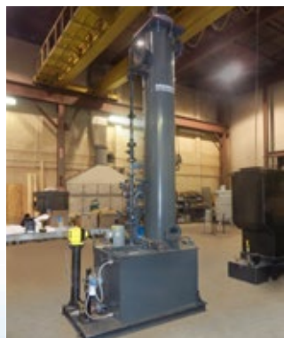
Amine Scrubber provides fume control: Packed Tower Scrubber for a gulf coast chemical manufacturing plant to control odorous fumes from chemical storage tanks.
