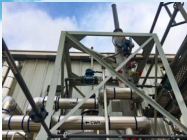
Two-stage Wet Scrubber with C-276 hastelloy Quench Tower and FRP Packed Tower to remove HF from gas stream at a chemical plant using KOH. The systems included integral scrubber sump, recirculation pump, piping, instruments, valves, and supports for hurricane wind speeds.
