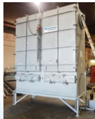
Fiber Bed Mist Collectors for asphalt storage terminal to control PM 2.5 particulate, fumes, mist, and vapors exhausted from its heated asphalt storage tanks. Downstream H 2 S adsorption vessels would plug and fail if these pollutants were not removed. The mist and vapors were very fine, requiring filtration equipment capable of removing submicron particulate.
