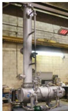
Wet Scrubber removes and recovers phenolic formaldehyde resin from nitrogen gas stream for a gulf coast chemical manufacturing plant.
