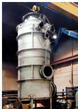
Evaporative Quench Tower for FGD project: Tower designed to ASME Section VIII pressure vessel standards.
