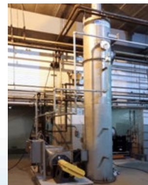
Air Stripper removes ammonia from ethylene glycol to increase the purity of the recycled liquid for an industrial solvents facility.
