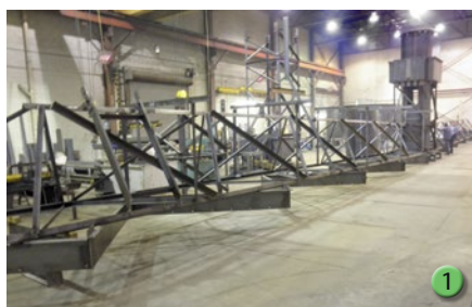
Before (Photo 1): Assembly of 130 ft. clarifier rakes
