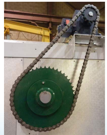
Drive and drive chain during shop testing
