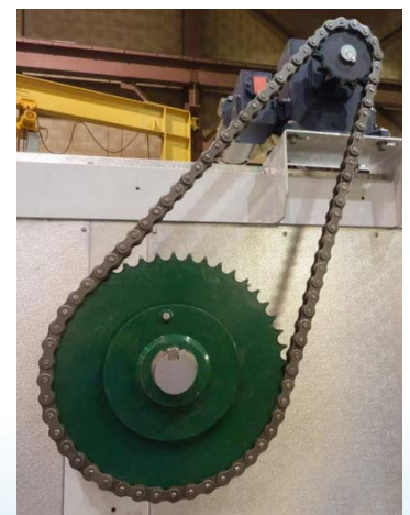
Drive and drive chain during shop testing
