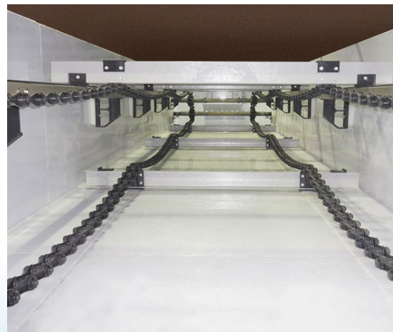
Chain and flight collector with non-metallic chain, flights, wear shoes, and flight supports.
