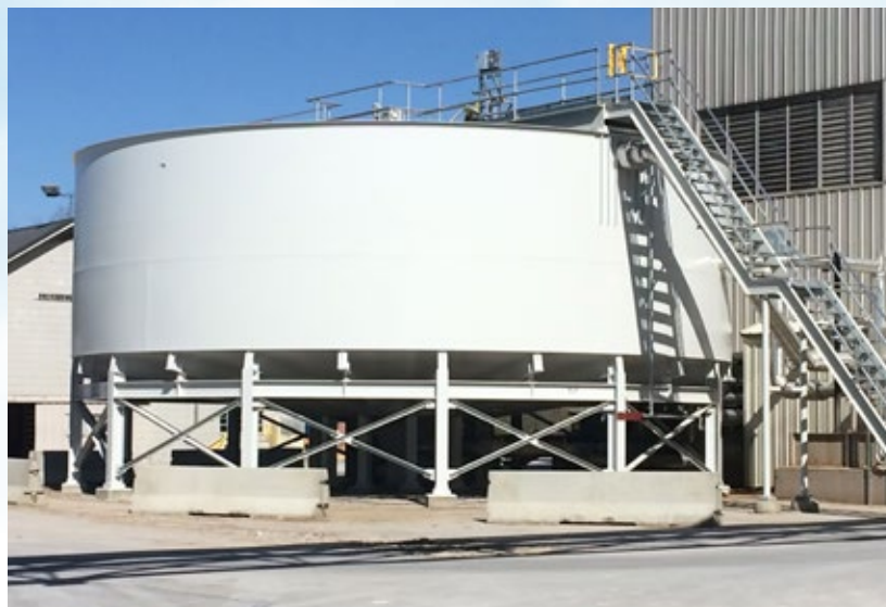
800 GPM Thickener Clarifier to separate dense, sticky solids contained in the liquid stream at a gypsum manufacturing plant. Solids are now properly agitated and pumped out in a timely manner, preventing material setting that had previously damaged equipment and stopped production.
