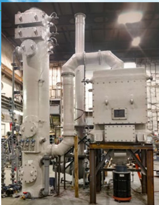
2,500 ACFM Multi-Stage Scrubbing System for PM and acid fume (HCl/HF) capture from building material testing oven prior to RTO. The system consists of a C-276 Quench Tower, FRP Dust Collector, Packed Tower Scrubber, pumps, instruments, and controls.
