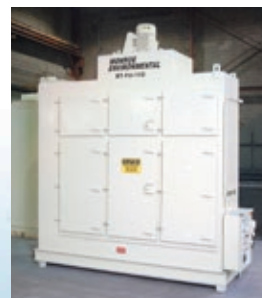
Multi-Stage Oil Mist Collector to remove heavy oil droplets, smoke, and submicron vapors for a synthetic fiber plant's manufacturing operations. The four-stage system operates at >95% efficiency treating 0.3 micron sized particles.
