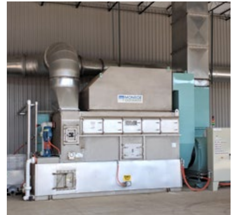
25,000 CFM Venturi Scrubber for aluminum parts manufacturer to upgrade their air pollution system. The scrubber effectively captures and removes lubricant mist, particulate, and fumes from their die casting process.
