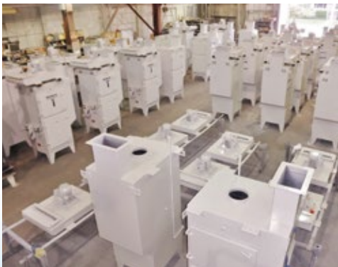
Assembly of 37 Spiral Tube Oil Mist Collectors for automotive engine and transmission machining operation. Monroe Mist Collectors outperform all other collectors and are currently operating at plants all around the world.
