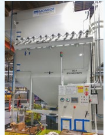
12,000 CFM Cartridge MQL Collector with integral fan and cartridge pulse controls at an automotive plant.
