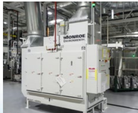
Multi-Stage Mist Collector with high efficiency filters and integral controls. Monroe's design incorporates more filter media than competitor units for longer operating cycles between filter changes.
