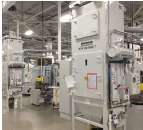
Cartridge Dust Collectors for dust filtration from grinding operation at an automotive manufacturing facility. Each unit is rated for 1,200 ACFM and features automatic reverse pulse cartridge cleaning and final HEPA filter to meet stringent emission limit.
