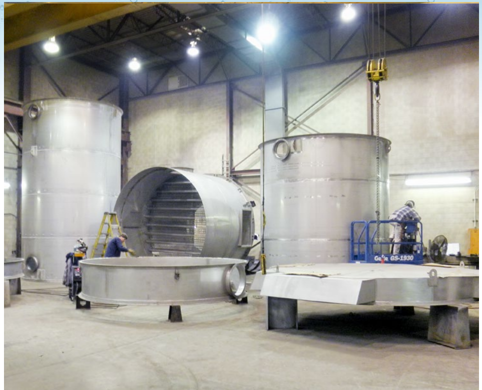
Air Stripper during fabrication at Monroe plant
