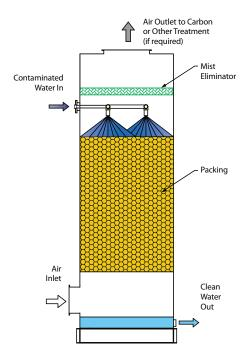
Packed Tower Air Stripper standard configuration
