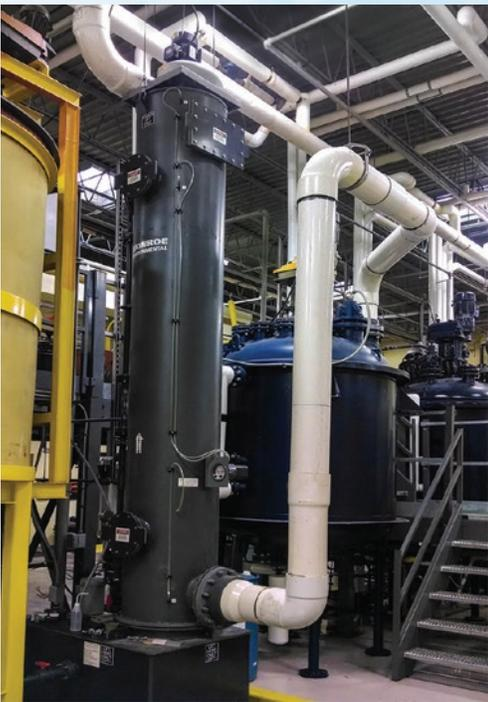
**Fume Scrubbing:** 1,200 CFM Packed Tower Scrubber, PVC construction with top-mounted fan for removal of iodine fumes from reactor tanks
