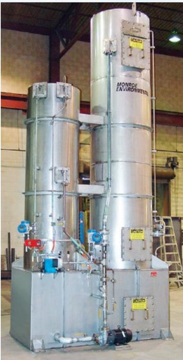
**Sulfur Dioxide Scrubbing:** SO<sub>2</sub> Scrubber with Quench Section and Packed Tower
