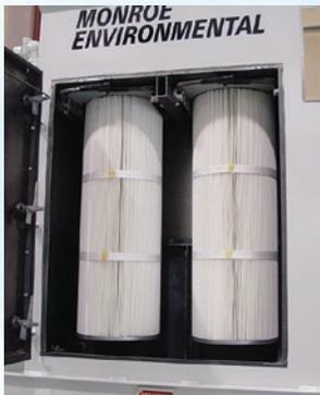
Vertically mounted, pleated fabric filters ensure high efficiencies for both dust collection and filter cleaning
