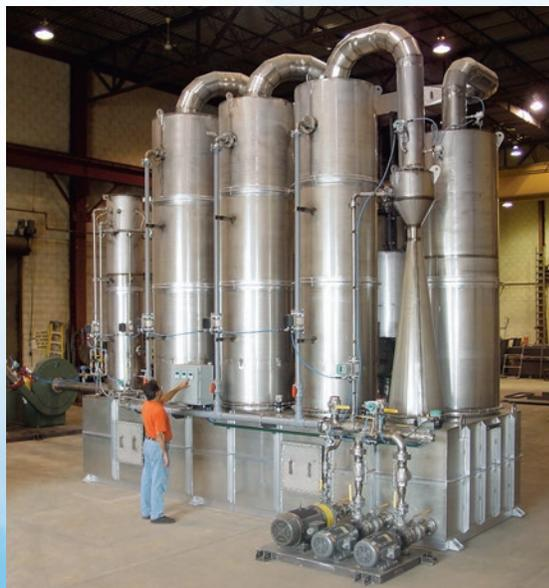
*Stainless steel Multi-Stage Scrubbing System to treat exhaust from a toxic gas incineration process*
