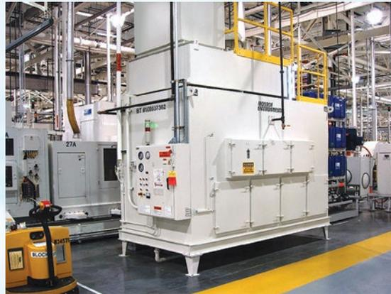
*Above: Packed Tower Scrubber for SO<sub>2</sub> removal from waste incinerator exhaust, 316 SS construction*
