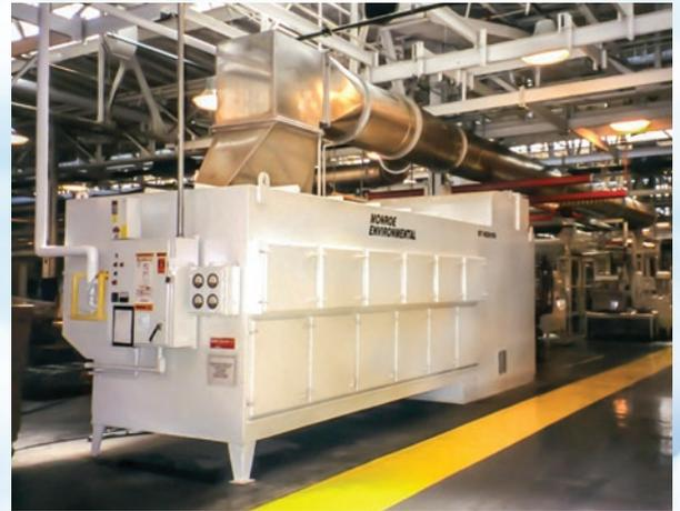
Monroe Mist Collector exhausting multiple machining operations at once
