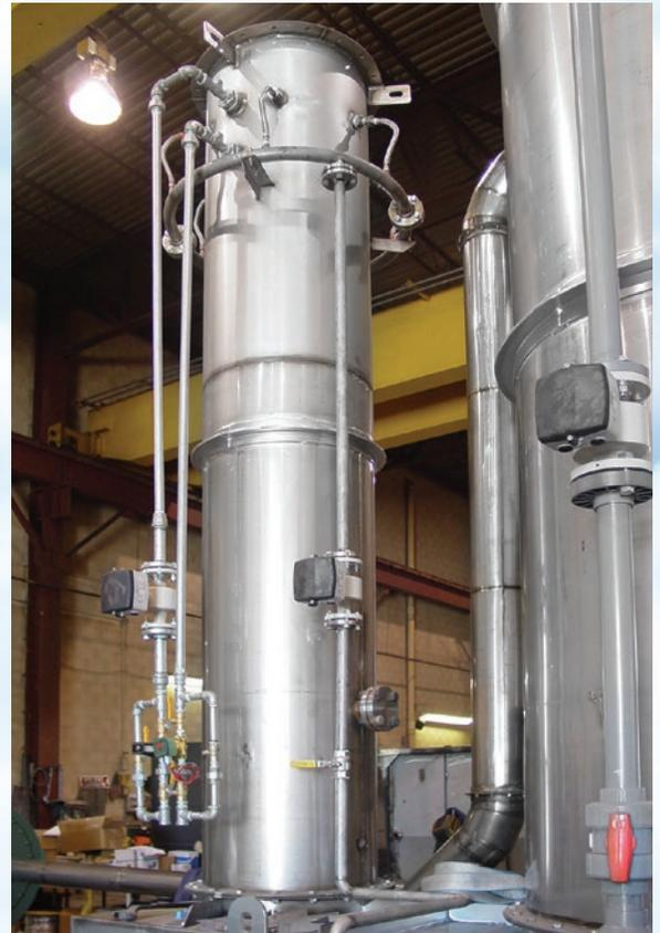
*High temperature and corrosion resistant evaporative Quench Tower*
