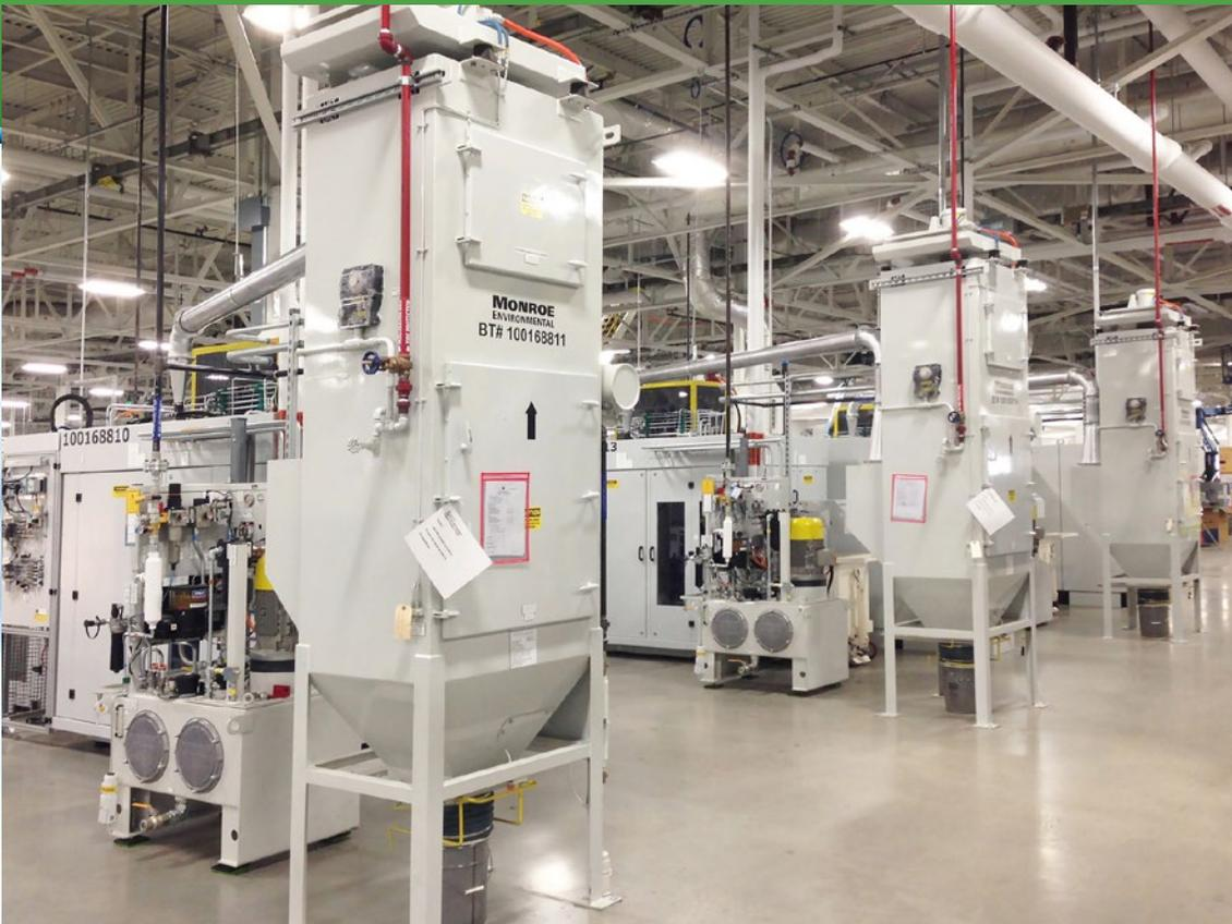
*Monroe Cartridge Dust Collectors equipped with fire suppression systems operating in the field*
