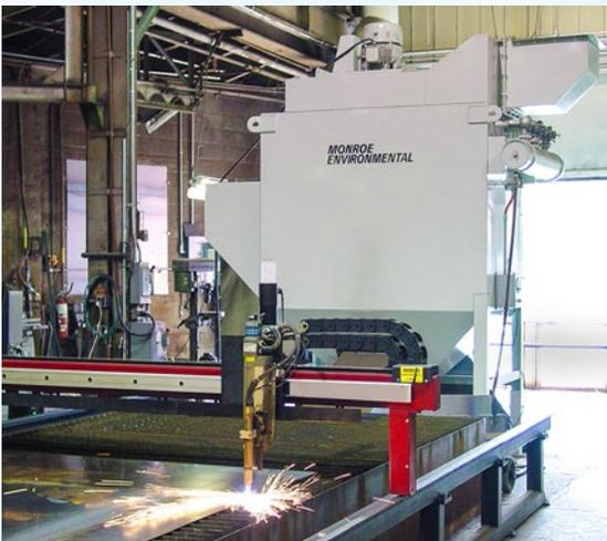
*5,000 CFM Cartridge Dust Collector to capture exhaust from a CNC plasma cutting operation*
