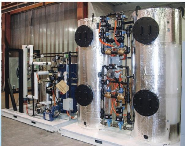
*High pressure scrubbing system to remove sulphur compounds from a propane gas supply*
