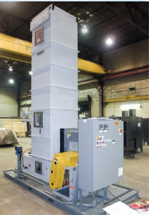
**5,000 CFM Packed Tower Scrubber,** polypropylene construction to remove acid gasses from chemical tanks at a recycling facility
