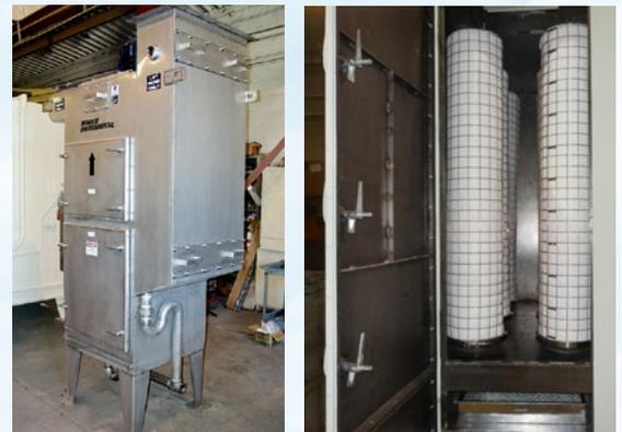
Left: 1,000 CFM Spiral Tube Mist Collector, stainless steel construction to filter mist from a washer at a food processing facility
