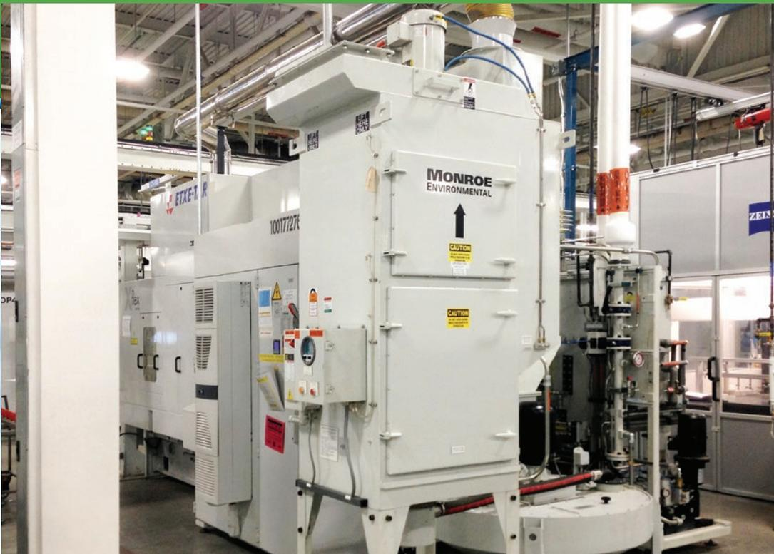
*Mist Collector exhausting a high production machining line at an automotive plant*
