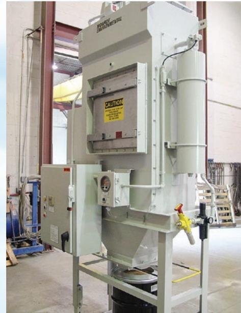
*Monroe Cartridge Dust Collector with explosion control system*
