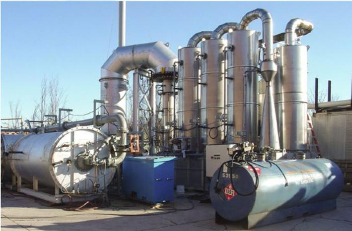
Multi-Stage Scrubbing system with inlet quench, 3-stage Packed Bed Scrubber, high energy Venturi Scrubber, electric gas reheater, and Carbon Adsorber for toxic gas incineration
