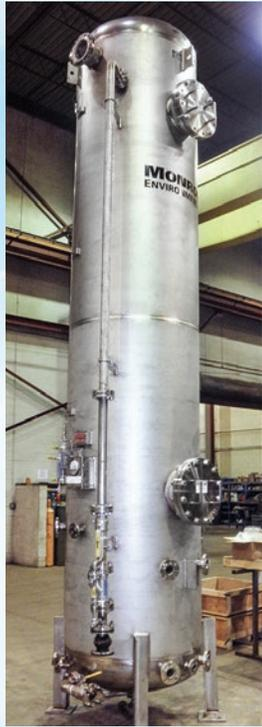
*Acid Gas Scrubbing: 1,500 CFM Packed Tower Scrubber, stainless steel pressure vessel construction to remove H<sub>2</sub>S from syngas for a diesel fuel conversion process*
