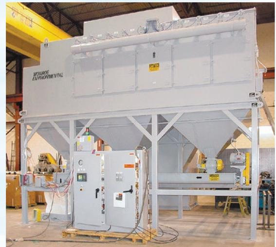
Custom configurations, including ceiling or roof designs, are available where a standard collector cannot be used. 30,000 CFM Dust Collector with multiple pyramid hoppers and screw conveyor options shown above.
