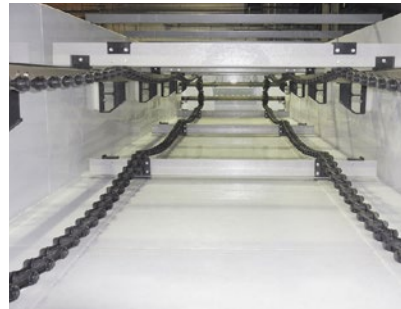
Left: (From left): Diffusion chamber with reaction jet baffles, screw conveyor for solids removal, and chain and flight drag conveyor. Middle: Chain and flight surface skimmer and drag conveyor in separation and settling zone. Right: (From left): Automated oil roll, adjustable pipe skimmer, underflow baffle, and adjustable overflow weir.
