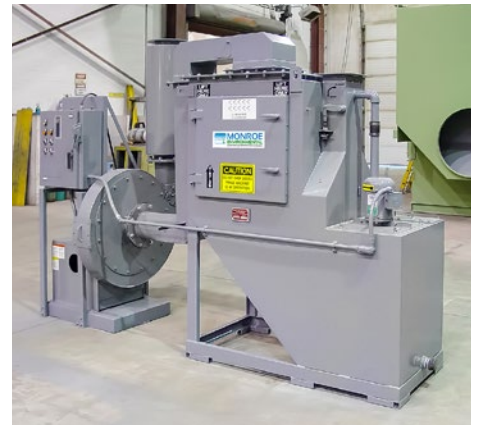
Venturi Scrubber and Cyclonic Separator for PM removal from dryer off-gas prior to RTO.
