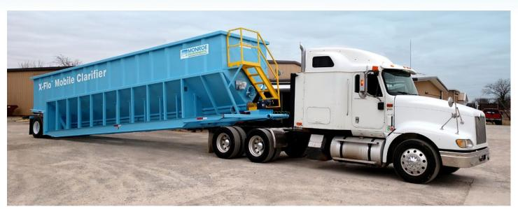
The **Monroe Environmental®** X–Flo™ Mobile Clarifier is a completely integrated mobile clarification solution for temporary job sites and/or bypass operations. The system can be utilized as a stand-alone clarifier or as a retrofit to improve the performance of existing mobile tanks.
