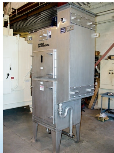
1,000 CFM Spiral Tube Oil Mist Collector, stainless steel construction to filter mist from a washer at a food processing facility
