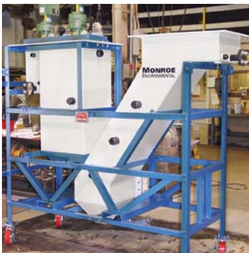
8 GPM polypropylene unit with chemical mix tank, flocculator, pyramid sludge hopper, and mild steel support structure
