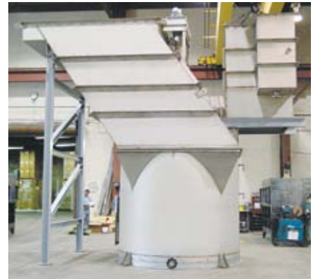
425 GPM stainless steel unit with chemical mix tank, flocculator, and thickener
