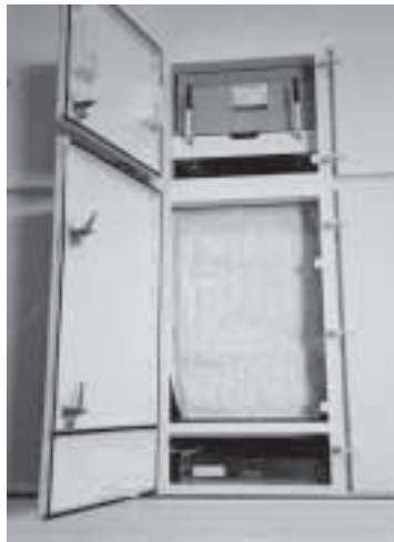
Open door showing separator screen element (bottom), fiberglass bag filter (middle) and HEPA filter (top).
