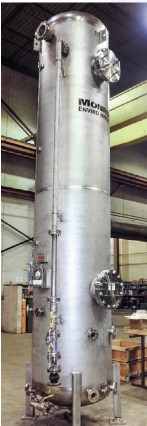
Acid Gas Scrubbing: 1,500 CFM Packed Tower Scrubber, stainless steel pressure vessel construction to remove H 2 S from syngas for a diesel fuel conversion process
