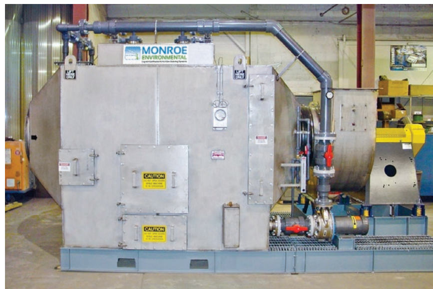
13,500 CFM skid-mounted Horizontal Packed Bed Scrubber, stainless steel construction to scrub acid and caustic fumes
