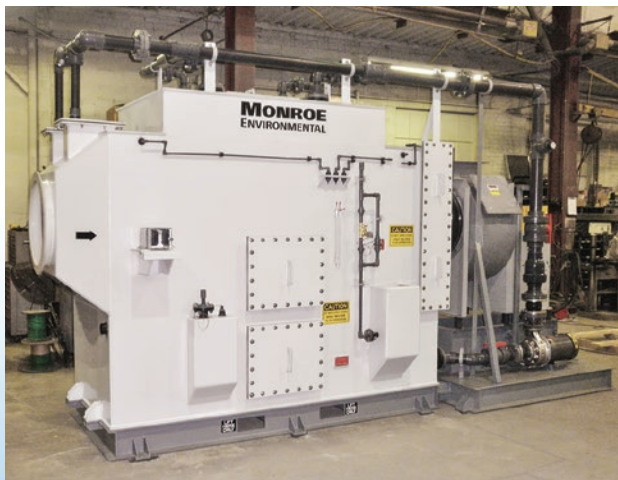
7,500 CFM skid-mounted Horizontal Packed Bed Scrubber, polypropylene construction to capture and remove NaOH fumes from kiln exhaust
