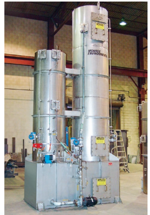
Sulfur Dioxide Scrubbing: SO 2 Scrubber with Quench Section and Packed Tower
