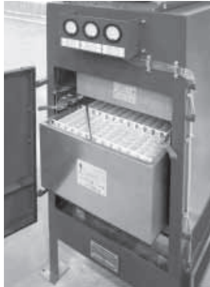
Open door showing separator screen element (bottom), fiberglass ASHRAE box (middle) and HEPA filter (top).
