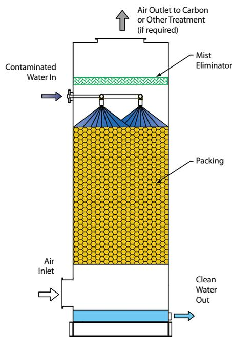
Packed Tower Air Stripper standard configuration
