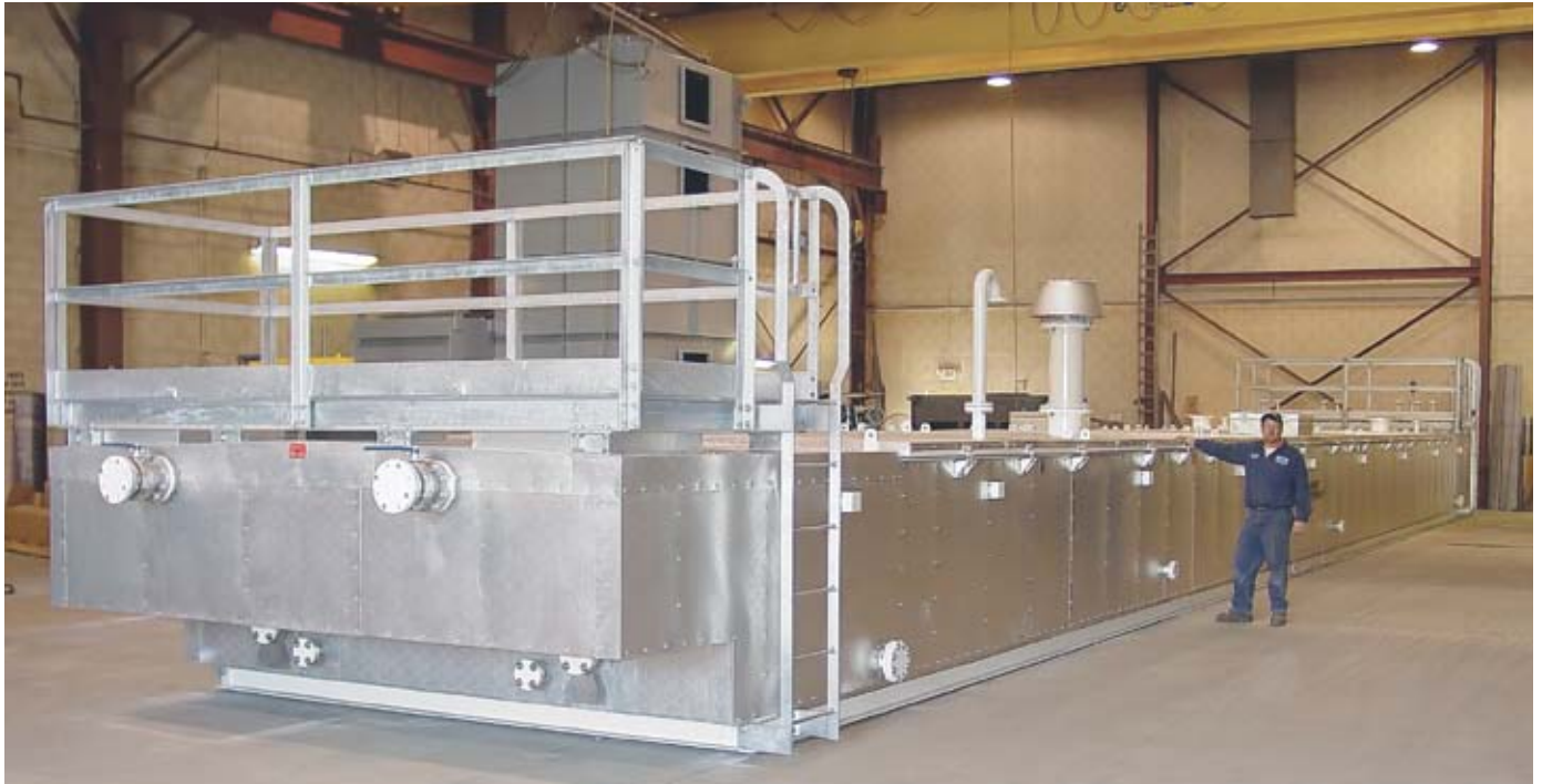
14 ft. x 90 ft. long 105 GPM API Separator with cover, insulation, and aluminum cladding. API Separators as large as 14 feet wide x 100 feet long can be shipped from our factory in one piece fully assembled.
